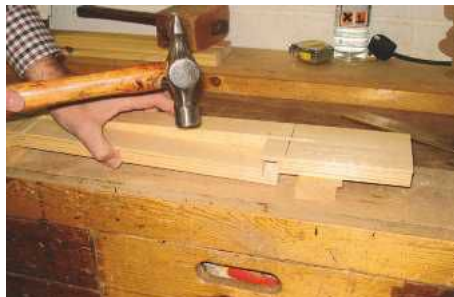
▲ Pic.8 After cutting with the gents saw, turn the work over and give it a sharp tap to free the pocket
